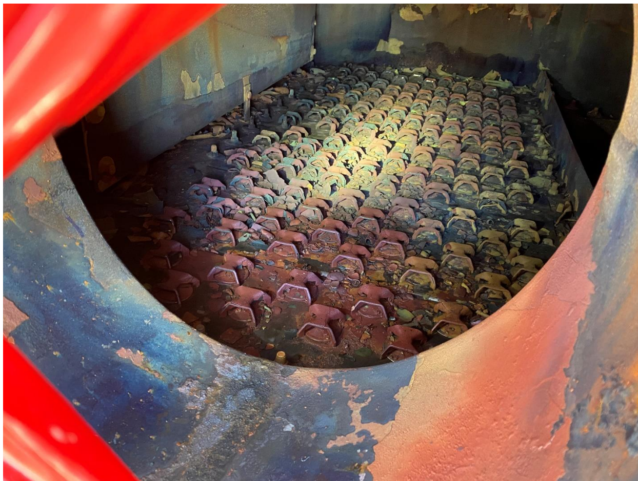
Figure 4: Amine Regenerator tray after a chemical cleaning fail
