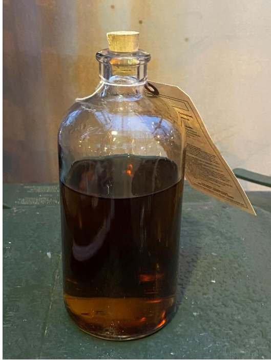
Figure 1: Amine solution turns brown after 12 hours of stripping for shutdown purposes
